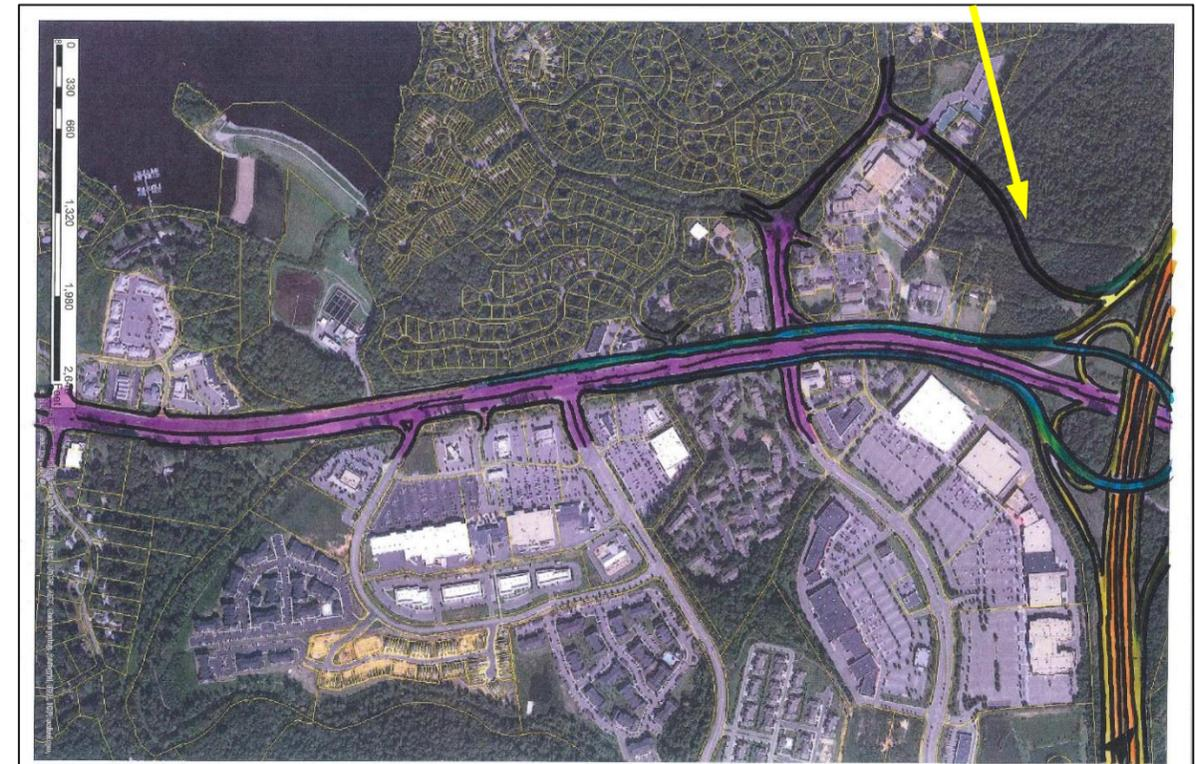
Figure 16: Concept #19 – Cloverleaf Interchange with Collector-Distributor (C-D) Roads
