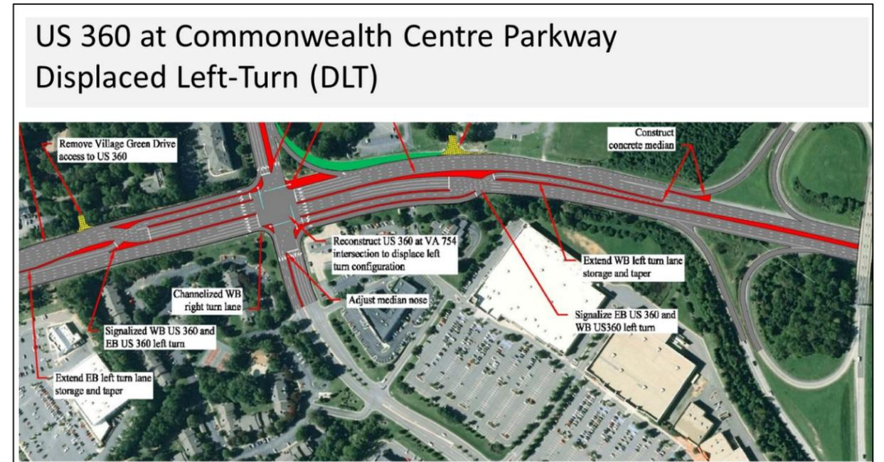
Figure 19: Concept #25 – At-Grade Displaced Left-Turn (DLT) Intersection with Additional Capacity
