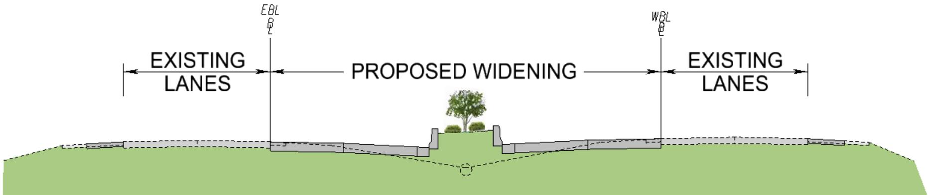
**This typical section applies to existing sections with a 64' median and bifurcation greater than 6"**
