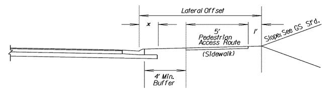
FIGURE A2-2 CURB WITH BUFFER STRIP AND SIDEWALK – CASE 2
