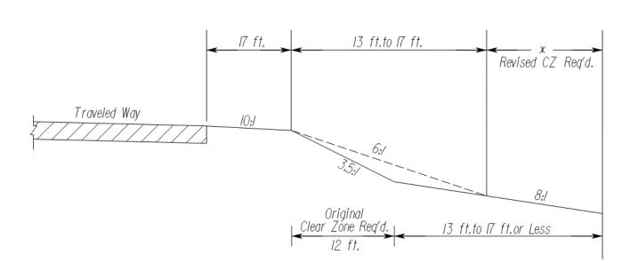
FIGURE A2-9 EXAMPLE OF ALTERNATE DESIGN INCORPORATING MINOR SLOPE ADJUSTMENT TO REDUCE TOTAL CLEARANCE REQUIREMENT
