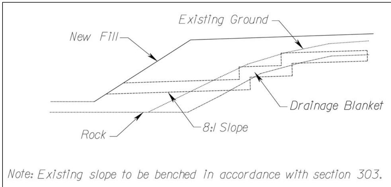
Figure 1: Rock Drainage Blanket Detail for Nondurable Shales
