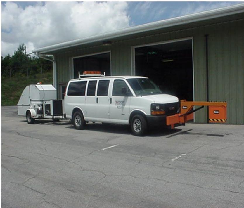
**Figure 3 - Falling Weight Deflectometer**
