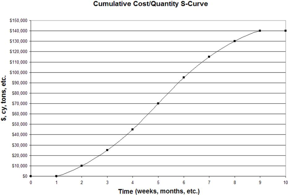
**Figure 2: Typical S-Curve**
