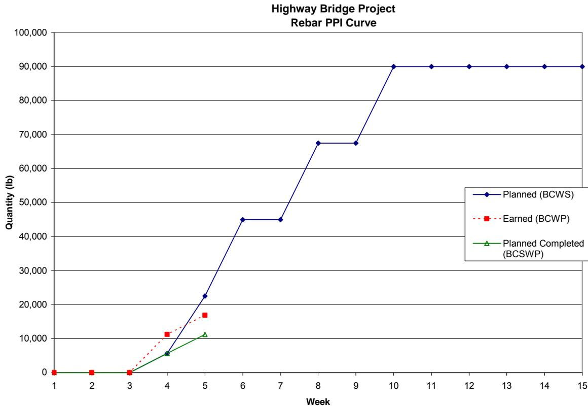
**Figure 16: Highway Bridge PPI Commodity Curve for Rebar**
