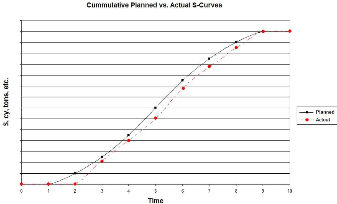
**Figure 3: Typical As-Planned versus As-Built S-Curve**
