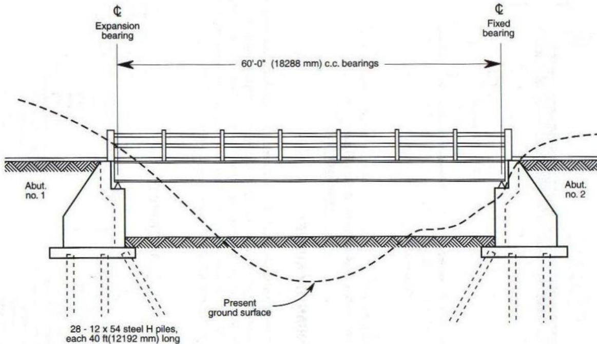
**Figure 5: Highway Bridge Profile (Clough et al. 2000)**
