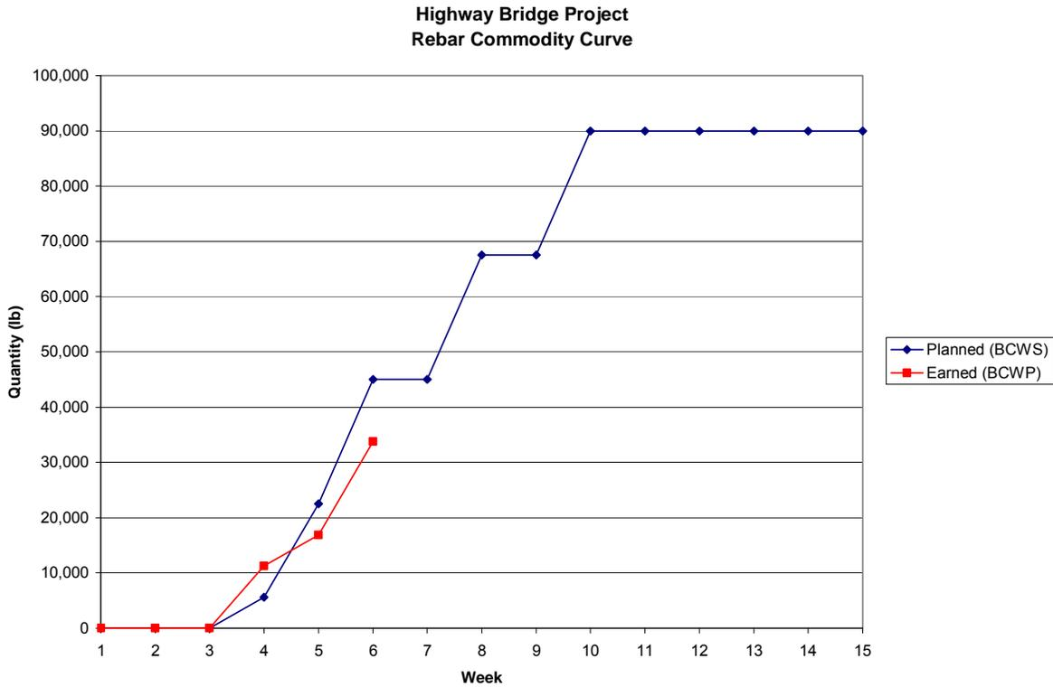
**Figure 12: Commodity Curve for Rebar in Week 6**
