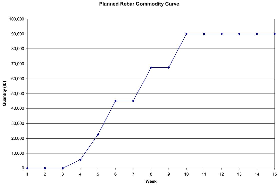
**Figure 8: Commodity Curve for Planned Rebar Progress**
