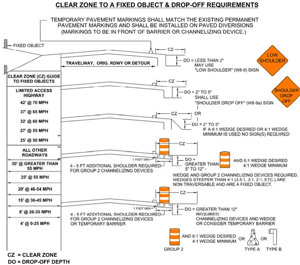
**Slopes steeper than 4:1 are considered a fixed object hazard.**
