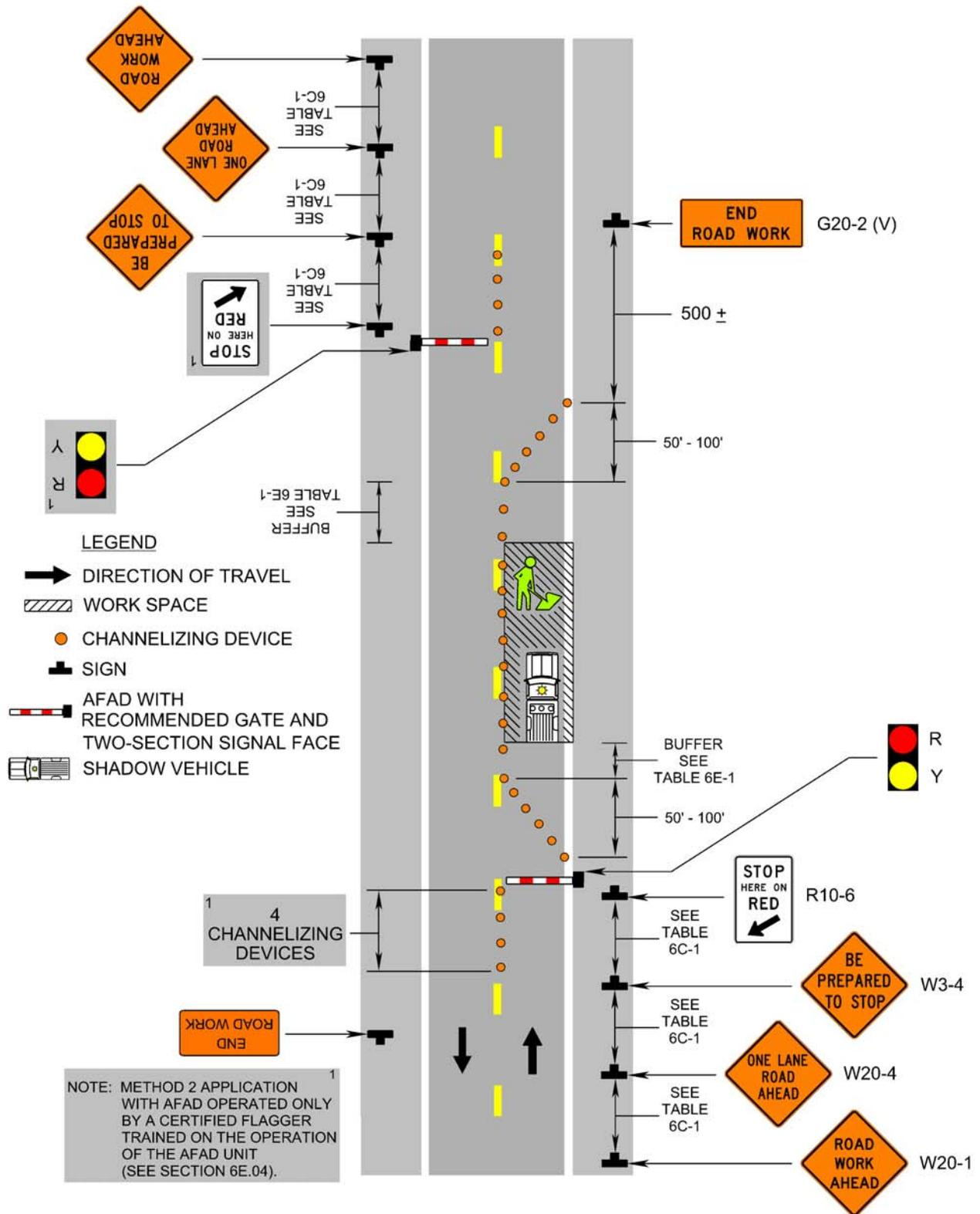
**Figure 6E-3, Use of Hand Held Signal Devices**
