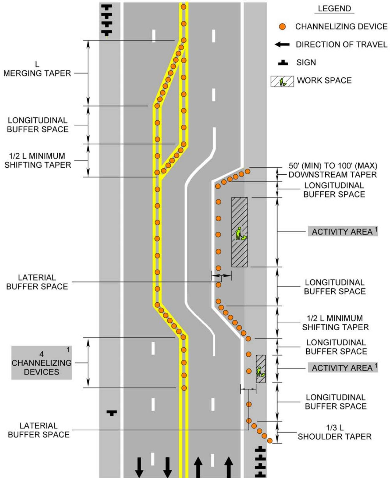
Figure 6C-3, Example of a One-Lane, Two-Way Taper
