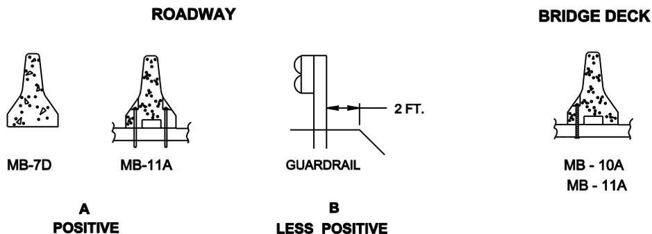
Barrier may require anchoring to the pavement or bolting to the bridge deck. Refer to Section 3, Barrier Design Considerations, for additional guidance. If anchoring/bolting is required it shall be on the traffic side(s) of the barrier. All barriers shall be installed in accordance with Section 500 of the current Road and Bridge Standards.
