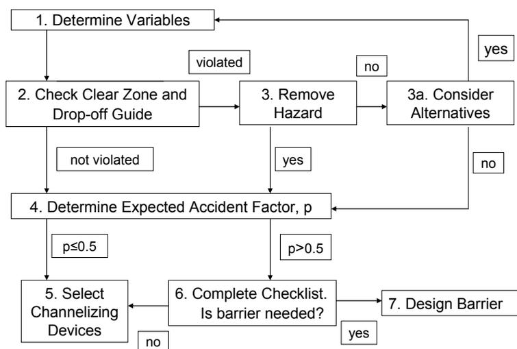
**Figure 2, Clear Zone and Drop-Off Requirements**
