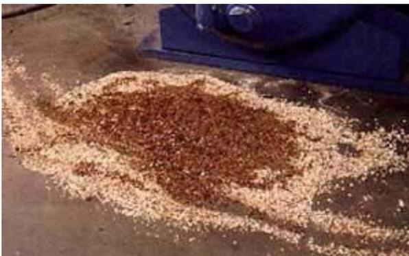
Oil absorbent used to clean up an oil spill
