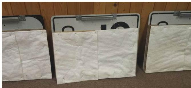
Oil absorbent pad attached to wood strips on old signs
