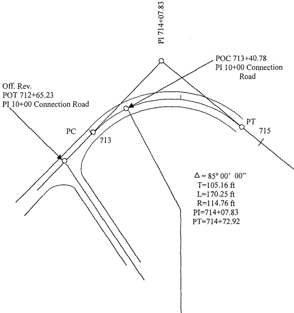
Check the notations on this plan and note that the original baseline for the connection at sta. 713+50.78 was a POC (Point on the Curve); however, subsequent revisions placed the actual connection to a POT (Point on the Tangent) at sta. 712+65.23.
