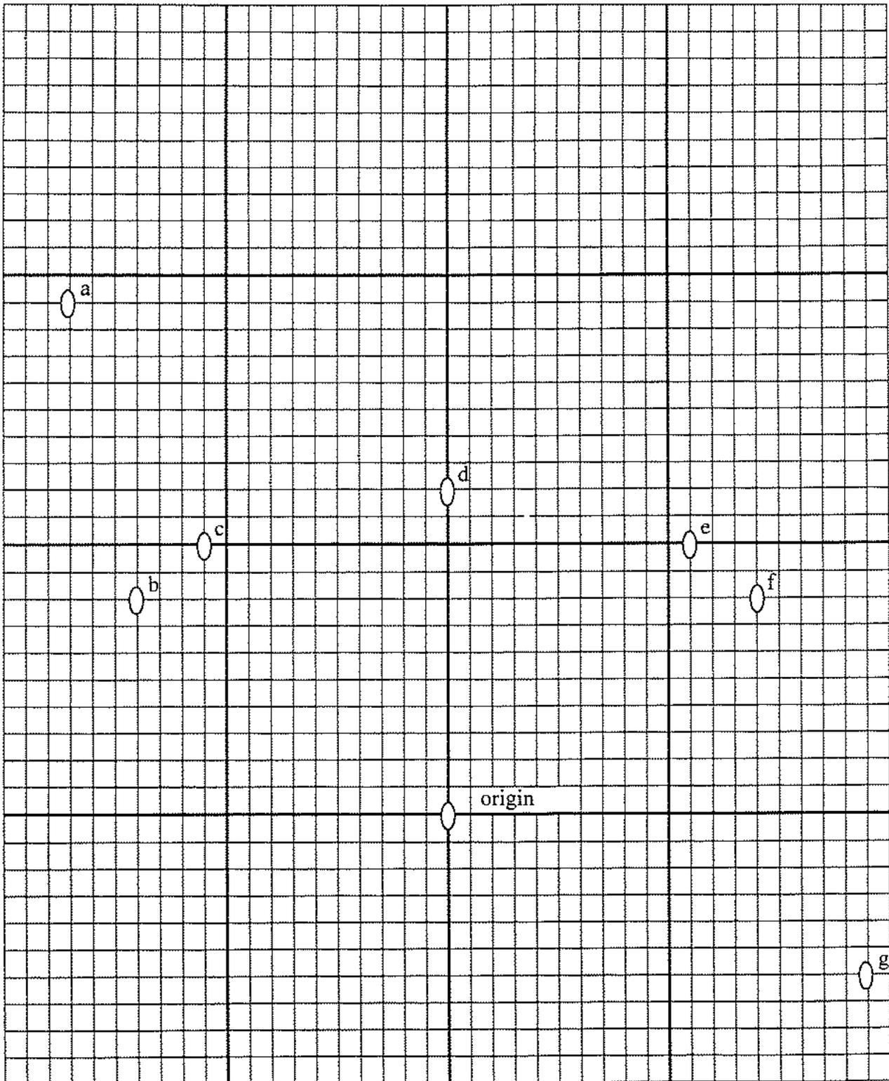
On this drawing, are several points labeled a, b, etc. Each of these points can be described as a distance or elevation vertically above or below or a distance horizontally right or left from the origin. These distances can be feet (or Elevation) above (or below) the origin and feet (Distance)
