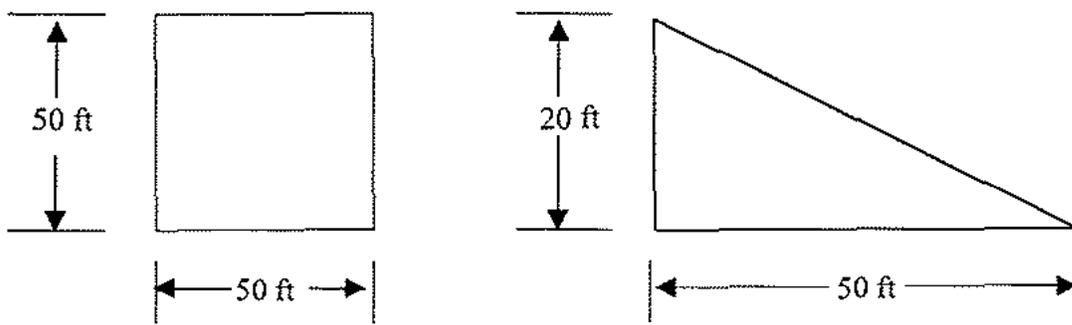
By now you should understand the exaggeration of dimension (measurement) found on the vertical (up and down) part of the Profile. Because of bumps and curves along the grade, which may be extremely small and hard to see, it is necessary to enlarge these by "blowing them up" so they can be readily seen.
