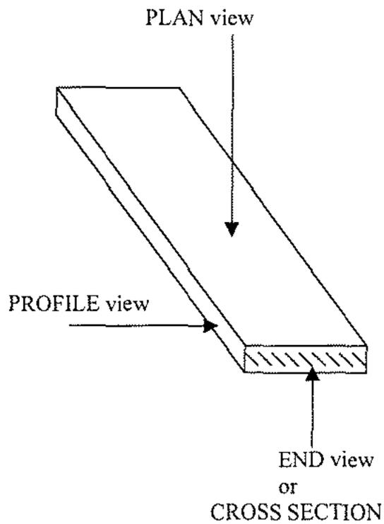
Here you see the Plan view, Profile view and the END view or CROSS SECTION.
