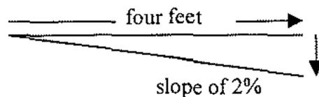
If you were four feet horizontally from the POINT OF FINISHED GRADE at the BASELINE, where the elevation was 10 ft, the elevation of where you are now would be 4 ft times 2% = 0.08 ft lower than the 10 ft elevation.
