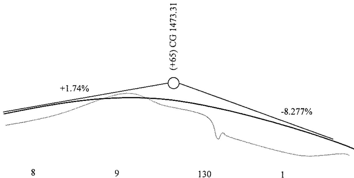
This drawing is a profile of existing and planned grades between stations 128+00 and 131+00. By matching this with a grading diagram you can see another view of what is happening. One point to remember is that the planned profile is at the baseline of the roadway. High or low spots to either side of baseline are expected and the grading diagram takes this into consideration.
