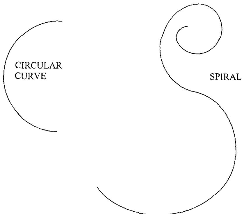
A circular curve would make a complete circle if it kept going around. A spiral curve would keep getting smaller and smaller if it kept going around. In order to approximate the path a vehicle makes when entering or leaving a circular horizontal curve, a spiral transition curve will be provided for horizontal curves with a radius less than or equal to 2865 feet, except for interchange ramps and loops.
