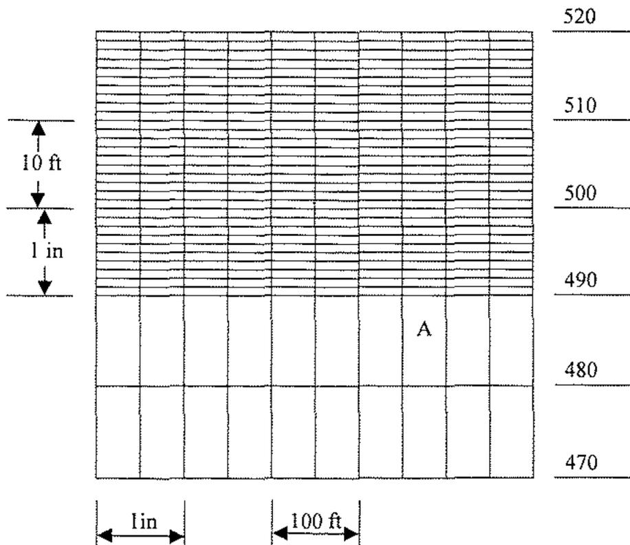
Study this drawing and determine the horizontal and vertical dimensions of block "A".
