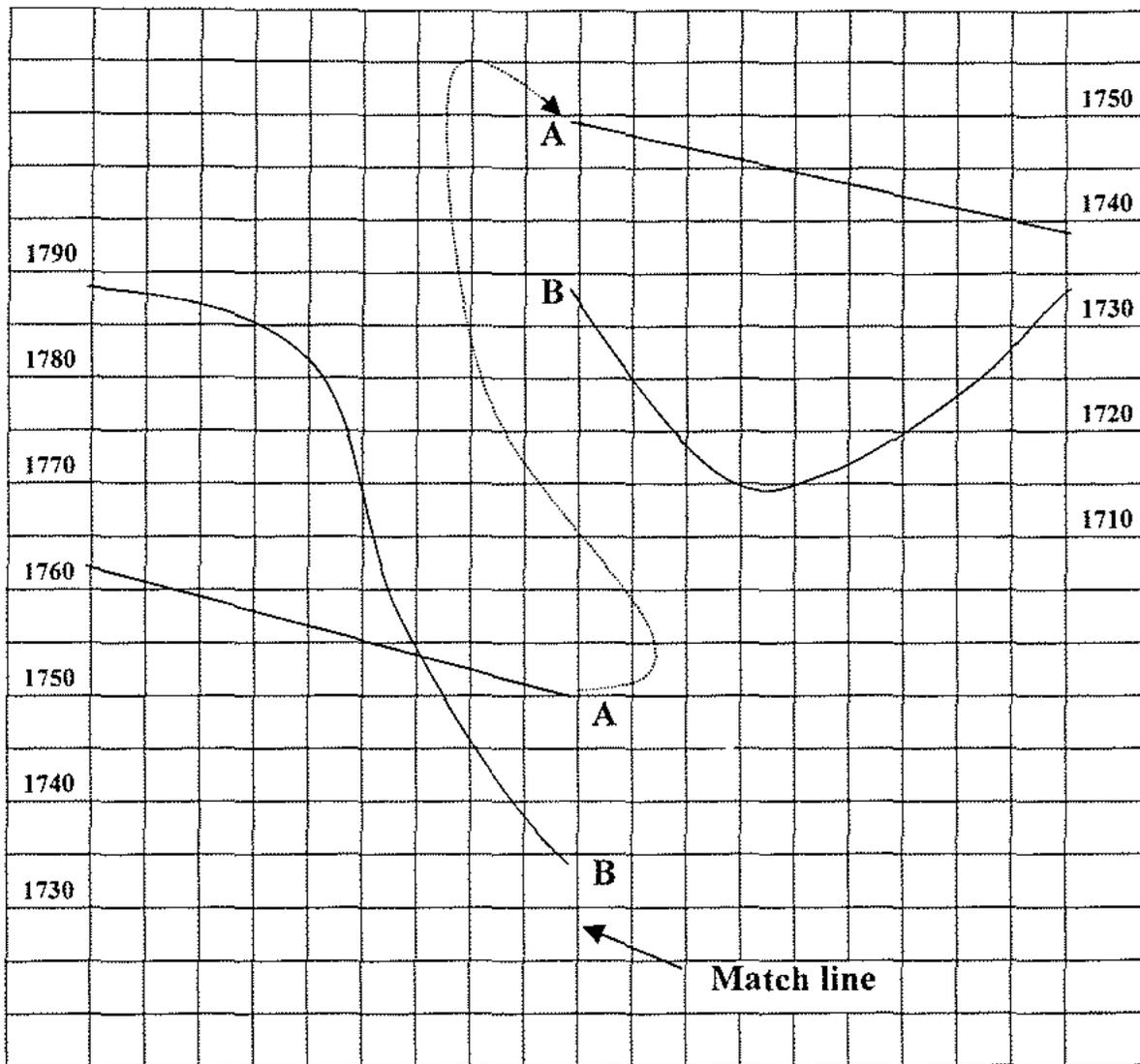
This partial profile illustrates a break in both the existing grade line and the proposed grade line. Notice that the vertical scales differ from side to side. The reason for this break is that the profile is too steep to illustrate it on our profile sheet. Therefore, we must raise the lower portion to fit within our limits. But to do this we must still have a scale by which to determine the elevation, thus we raise the lower scale also.
