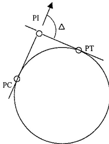
Δ This symbol is called delta, meaning delta angle, and refers to the angle between the original tangent direction and the new tangent direction.
