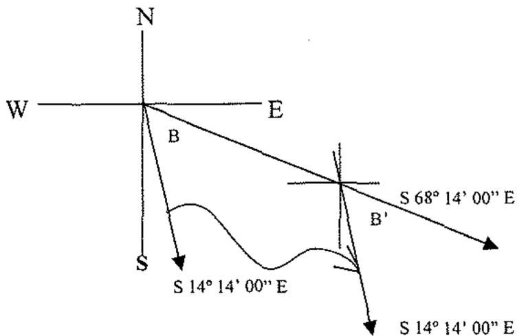
If we re-arrange our diagram by moving bearing S 14° 14' 00 E, tangents are formed and intersect.
