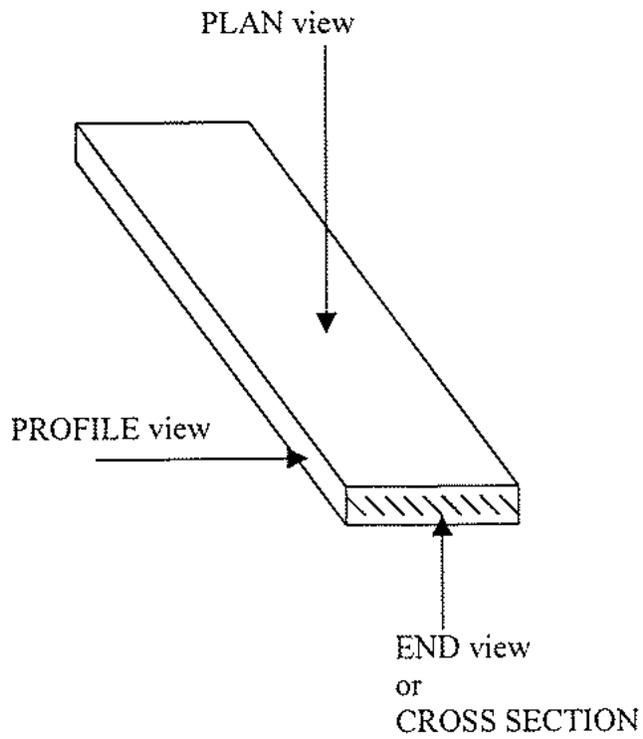
Here you see the Plan view, Profile view and the END view or CROSS SECTION.
