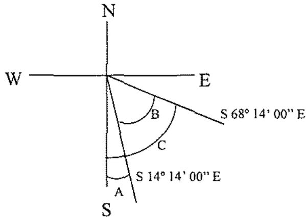
If we plot both of these bearings in the same manner, we find that angle A, formed between SOUTH and bearing S 14° 14' 00" E, is smaller than angle C, formed between SOUTH and bearing S 68° 14' 00" E.
