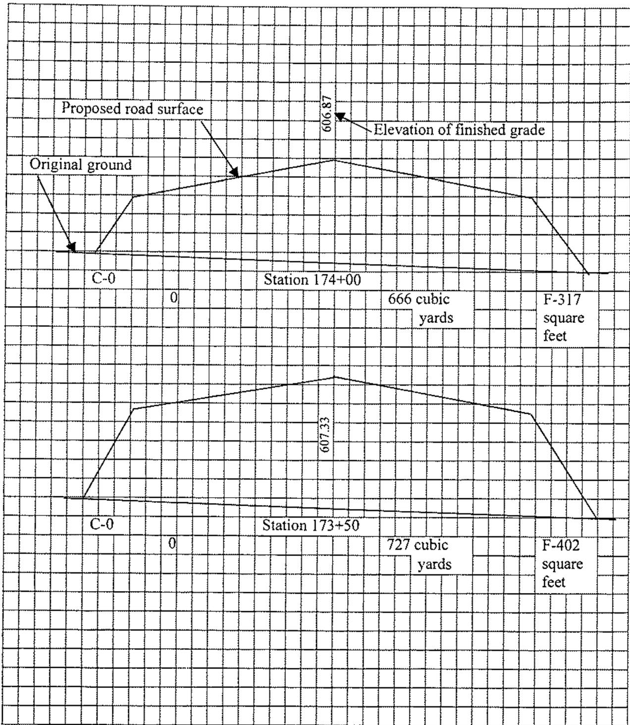
The previous drawing is of two cross sections taken at stations 50 feet apart. The lower section is taken at sta. 173+50.00. The Point of Finished Grade is at an elevation of 607.33 feet. The elevation of the existing ground is represented by the line that the typical section is resting on. These sections represent FILL sections along the project.
