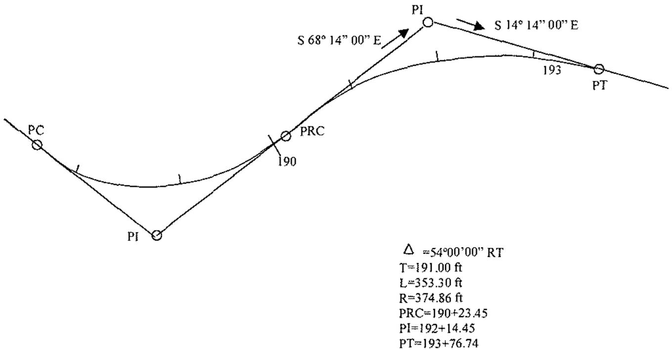
Check this drawing and note that the bearing of the tangent as it enters the curve (back tangent) is  $S 68^{\circ} 14' 00'' E$ . On the tangent between the PI and the PT (ahead tangent) a bearing of  $S 14^{\circ} 14' 00'' E$  is given.
