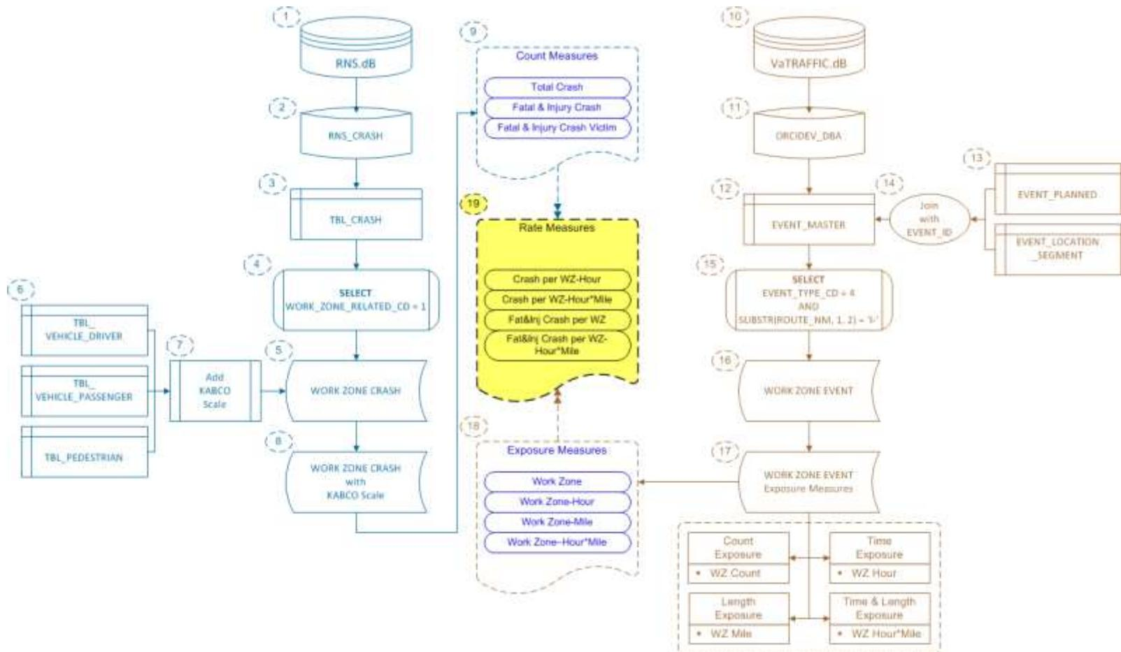
Figure D1. A Procedure of Calculating Measures of Work Zone Safety. Note that this procedure is executed for a year of interest for all roads in Virginia so that calculated measures are for Virginia in that year.
