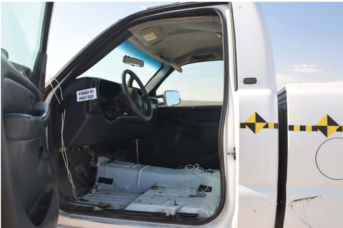
FIGURE 50. Post-Test Driver Side Occupant Compartment
