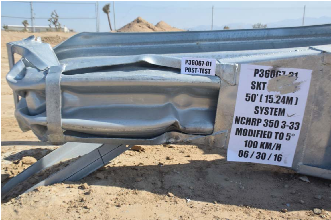
FIGURE 34. Test Article Damage
