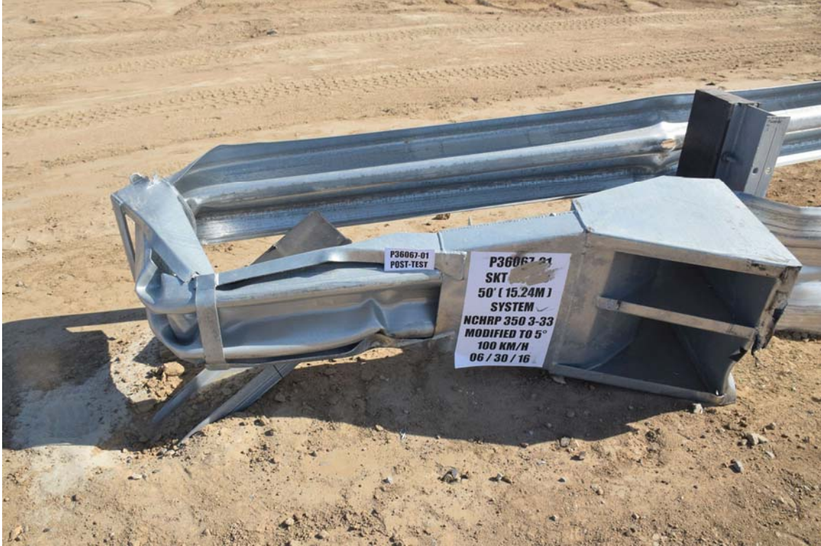
FIGURE 33. Test Article Damage
