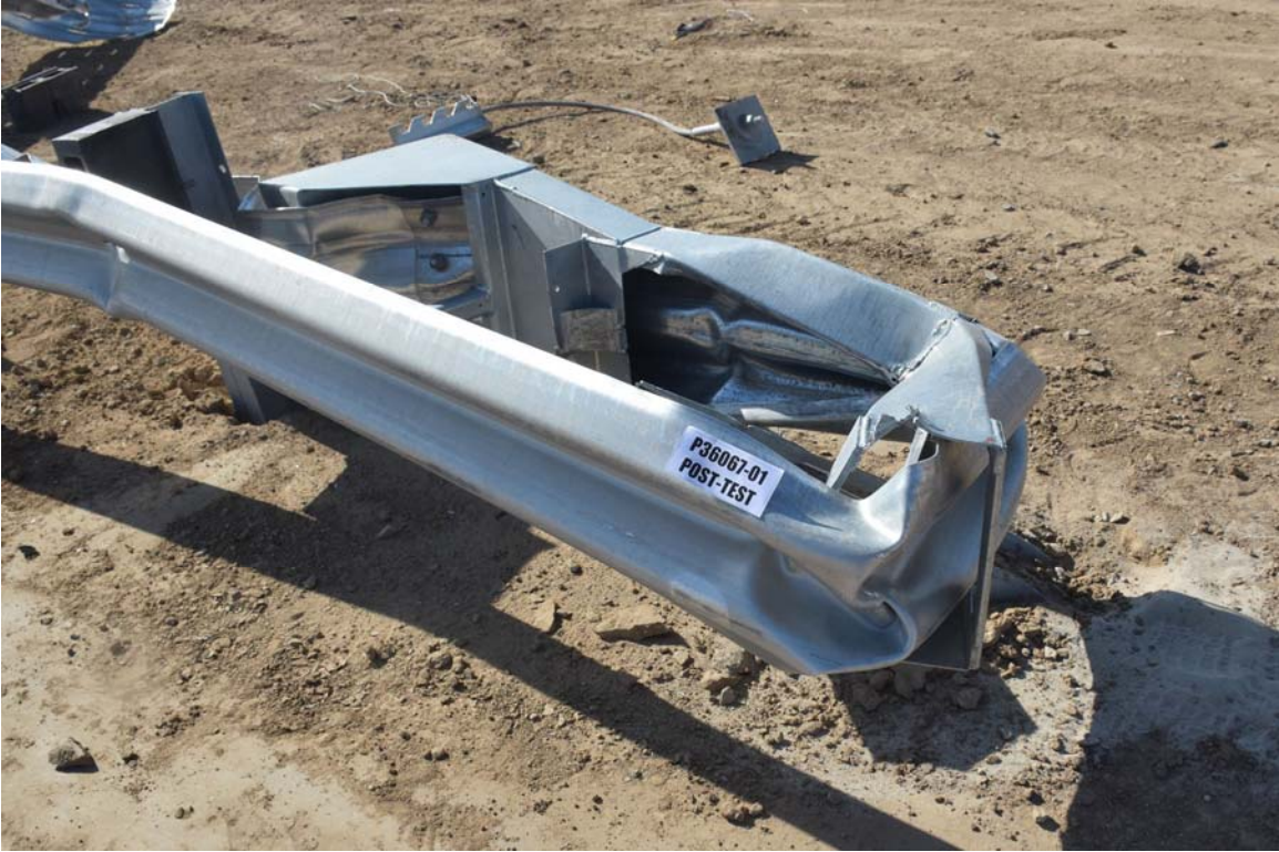
FIGURE 35. Test Article Damage
