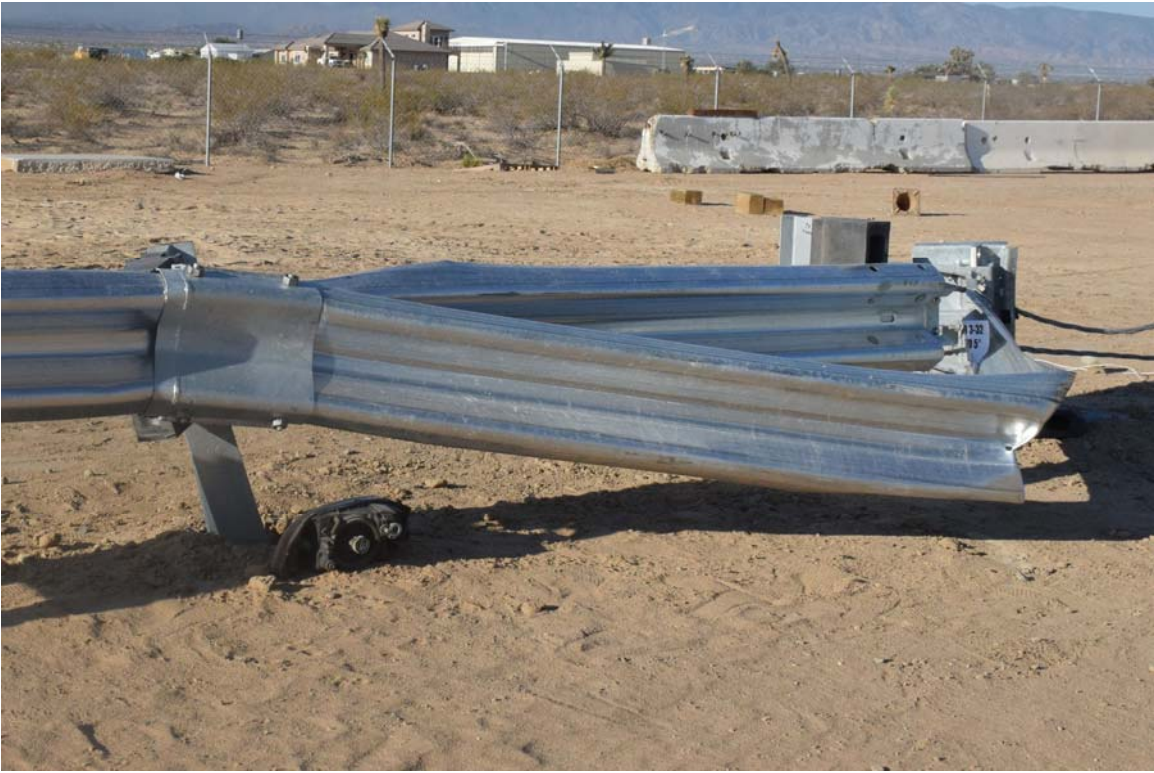
FIGURE 37. Test Article Damage
