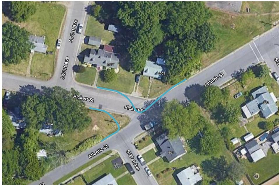
Figure 21. Sketch of intersection reconstruction, where blue lines indicate the new curb line
