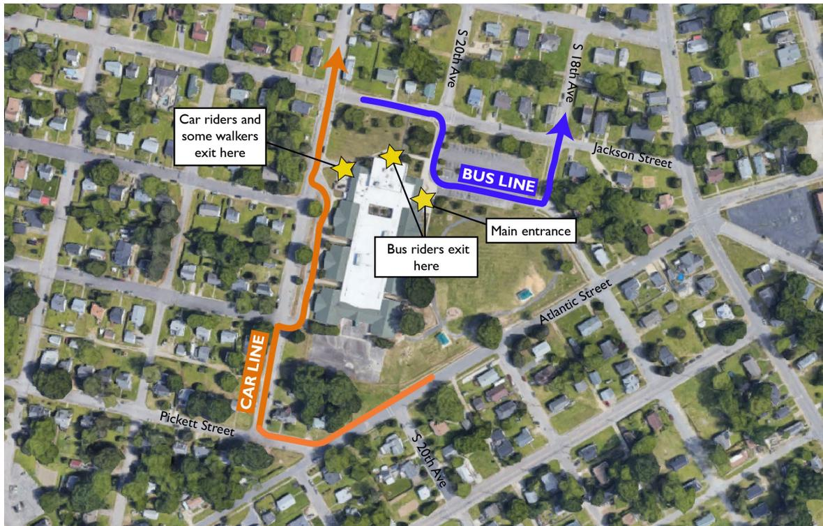
Figure 8. Car and bus circulation at dismissal
