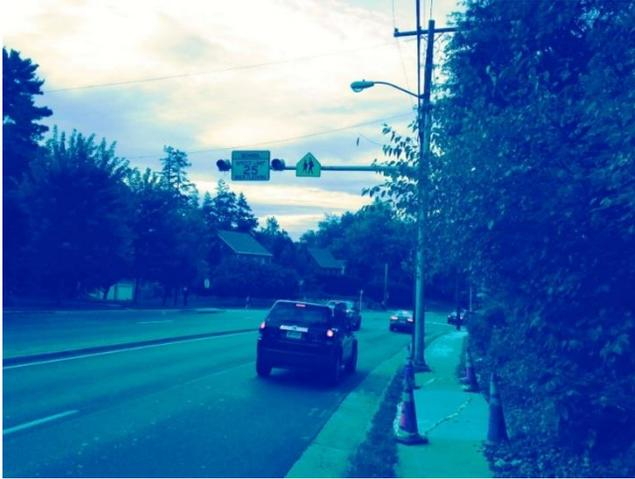
**Figure 6** The school zone speed limit sign and flashing beacon for southbound traffic is located on a curve approximately 350 feet north of the 18th Street N. intersection. This location has limited visibility for motorists and may not provide motorists with sufficient warning of the upcoming school crossing.
