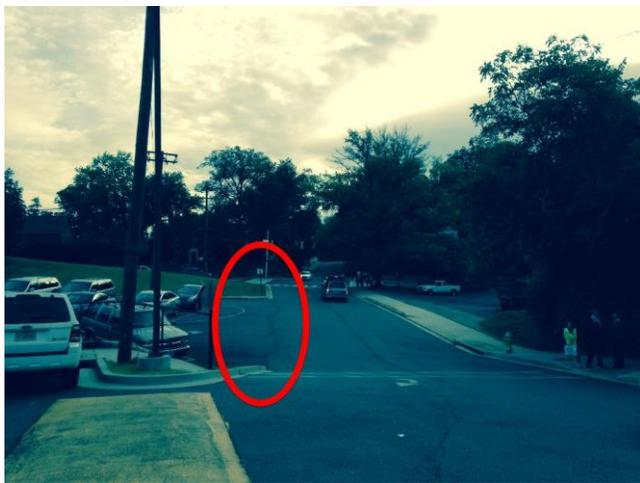
**Figure 9** There is no sidewalk on the school side of the school access drive. As a result, pedestrian must use the sidewalk on the south side of the school access drive and then crossover to the north side using the crosswalk at the entrance to the school parking lot
