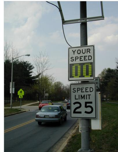
*Speed feedback devices display a driver's current speed next to the posted speed limit for comparison*
