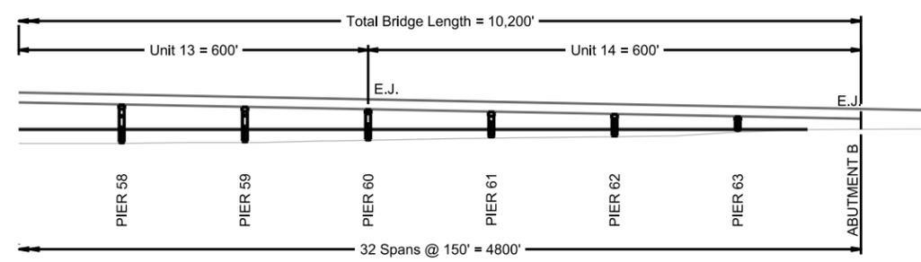
ELEVATION - PIER 58 THRU ABUTMENT B
