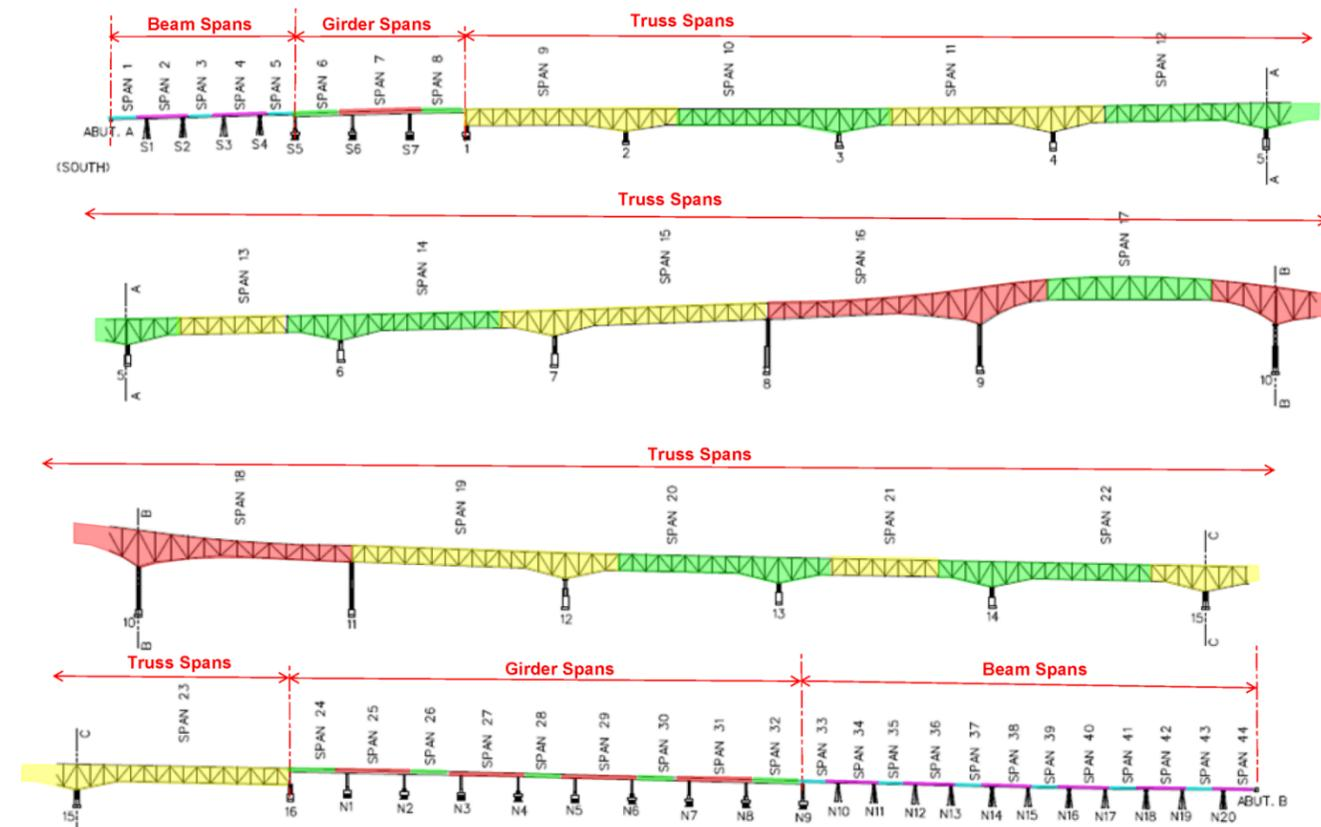
Figure 2-3: Existing Structure Configuration
