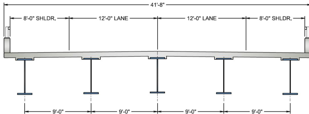
Figure 3-8: Multi-Beam Configuration – Option 2
