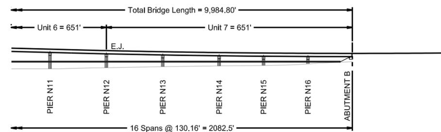
ELEVATION - PIER N11 THRU ABUTMENT B
