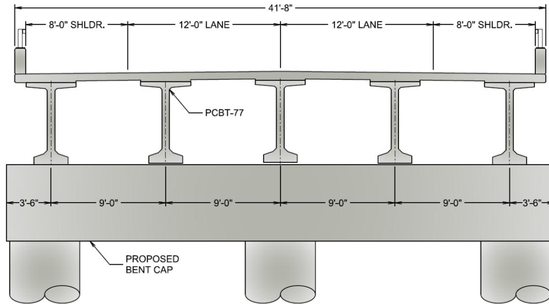
**Figure 3-10: Beam and Girder Span Section – Option 3**
