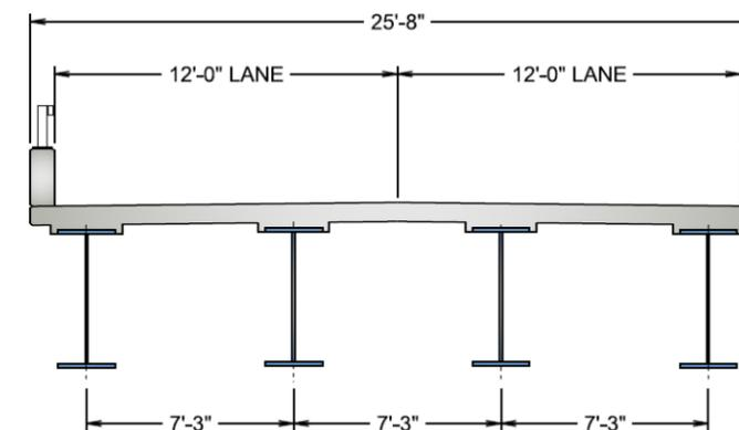
Figure 3-5: Beam Span Section – Option 1
