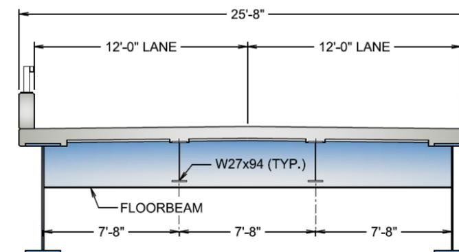
Figure 3-6: Girder Span Section – Option 1
