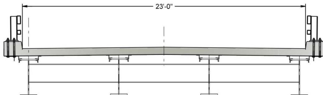
Figure 2-6: Existing Bridge Roadway Width (Beam Span Shown)
