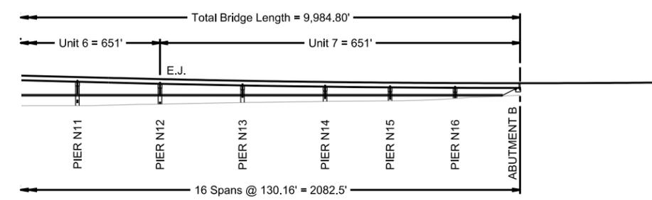
ELEVATION - PIER N11 THRU ABUTMENT B
