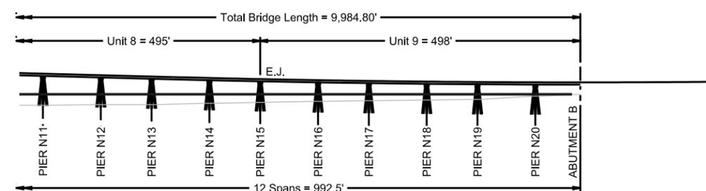
ELEVATION - PIER N11 THRU ABUTMENT B
