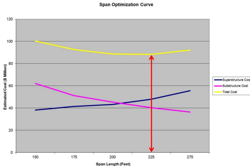
Figure 6-1: Typical Span Optimization Curve
