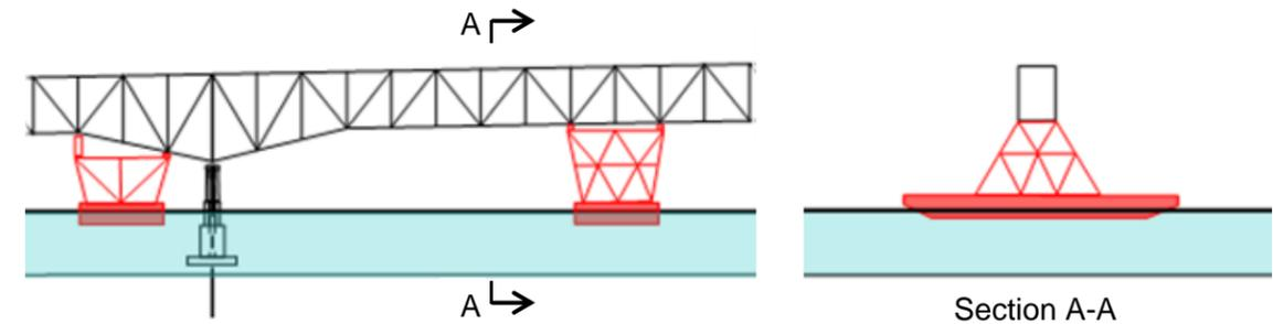
**Figure 4-1: Barge Configuration for Float Out**
