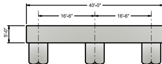
REPLACEMENT PIERS IN BEAM & GIRDER UNITS - SUPERSTRUCTURE REPLACEMENT - ALTERNATIVES B, C, D, & E
