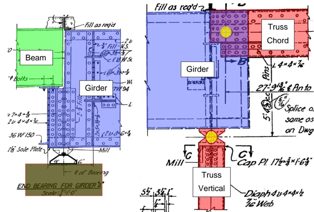
Figure 2-2: Girder Span End Conditions
