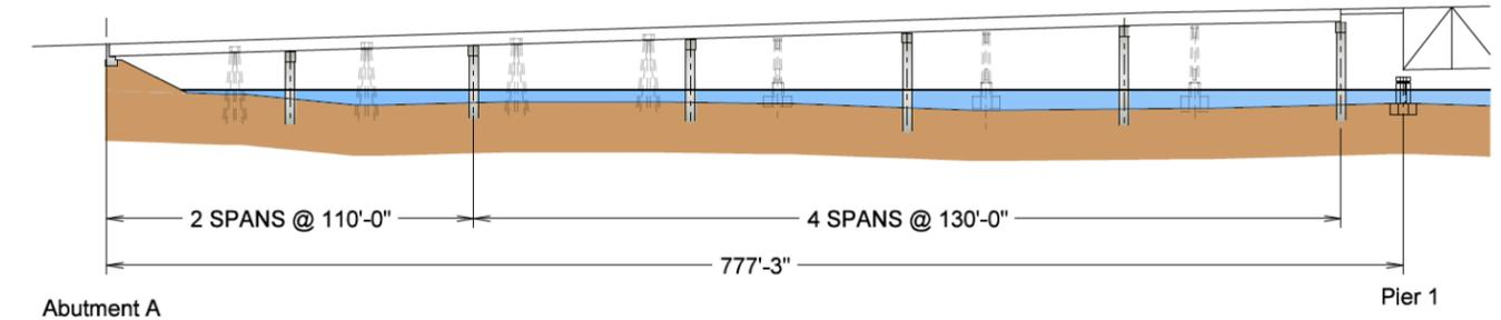
Figure 3-9: Potential New Span Arrangement (south approach shown)
