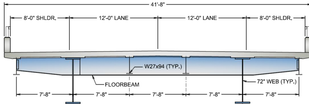
Figure 3-7: Two-Girder Configuration – Option 2
