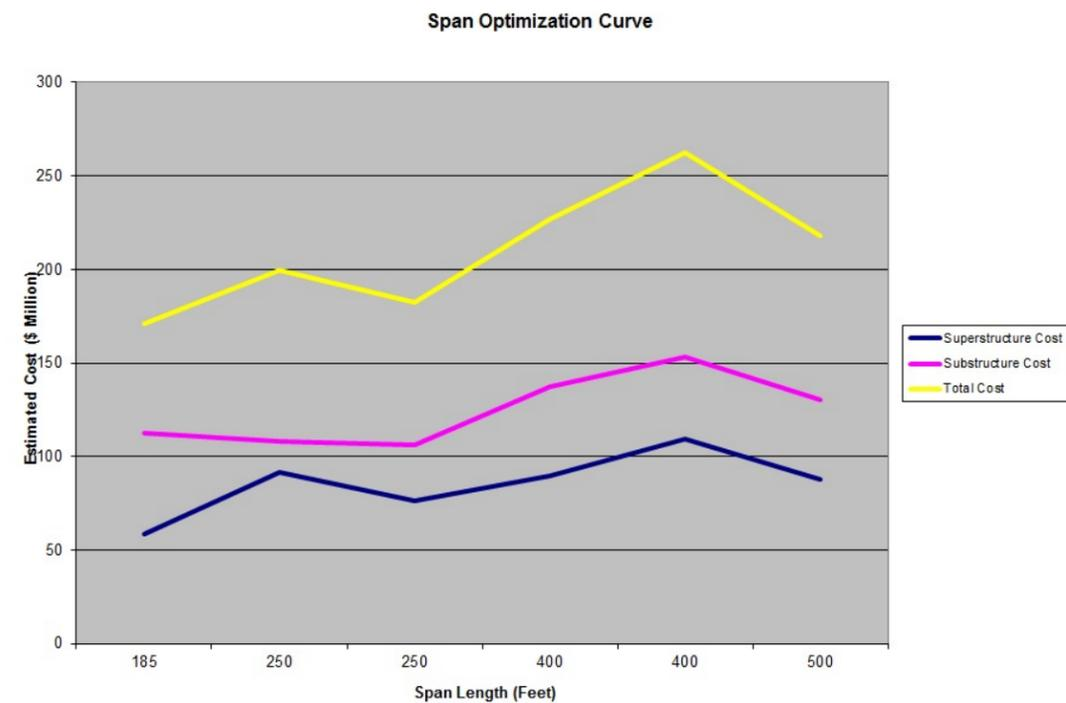
Figure 6-2: Route 3 Bridge Span Optimization Curve
