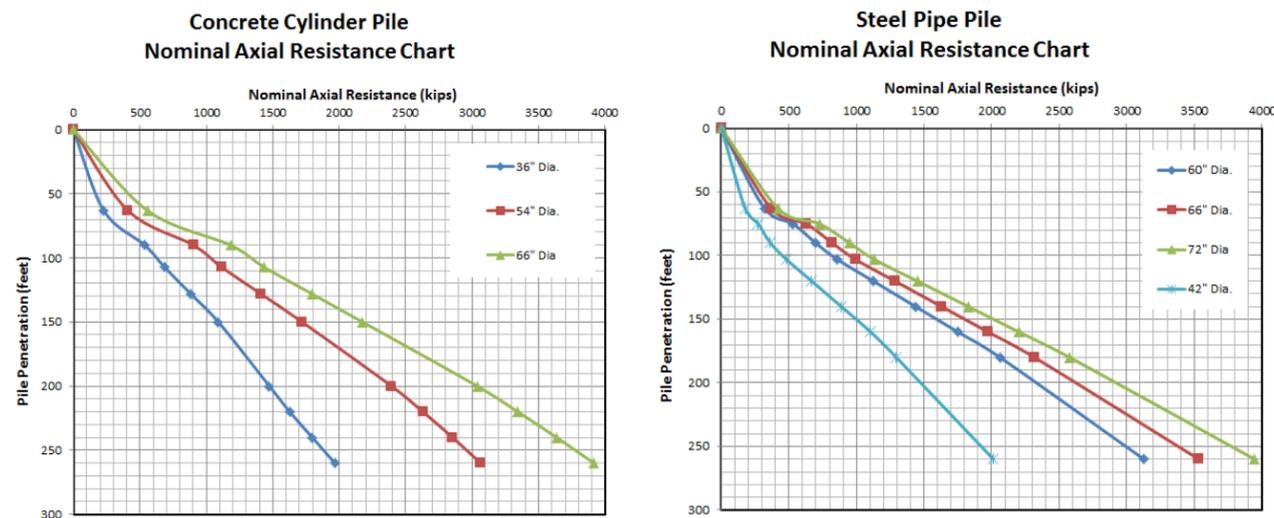
Figure 6-12: Idealized Nominal Axial Resistance Charts for Concrete Cylinder and Steel Pipe Piles
