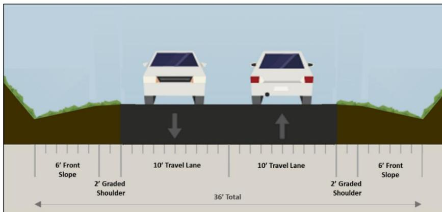
Figure 10: Rural Local Road Typical Section with Shoulders for Bikes
